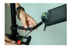
Regulate your position as you prefer, moving and pivoting the arm bracket, unfastening and fastening the screws with the regulation key
