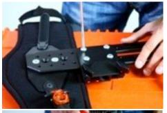
Regulate the right or left mating block poition. for example: if someone is using the sled with his right hand, he got to keep the mating block on his left side. Regulate the desidered height
