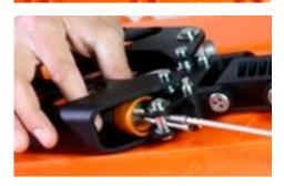
Now unfasten the 2 antirotation screws in the opposite side of the preload screws. Then extract the spring Repeat this operation for the other 3 springs.
