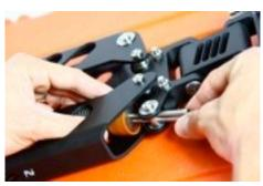
Insert the antirotation screws fastining till their end. Do not fasten hardly
