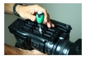
Fasten your camcorder with the 1/4" or 3/8" screws included in the kit, or fix the plate to your sony/ panasonic or other special plate. In case of camera not in axis use the lateral holes in order to balance in the center the camera's weight
