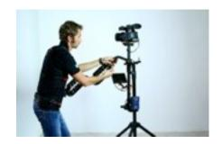
Now approach the sled on the docking plate and make a little squat on your legs to simplify the arm pin entering inside the sled handle
