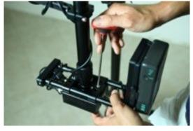
Unfasten the upper screws of the rod clamps, for positioning the battery pack in order to have the sled right balanced.
