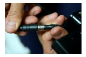
Connect the MINIDIN breakout cable, following the arrows for right connection
