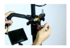
unlock the security pin Load all the weight and lift up all the system
