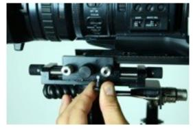
Attention: There's a security blocking pin wich avoid the accidental camera exit from the side to side. Pull down the pin during inserting or extracting your camera
