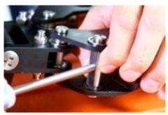
insert the long preload screws and keep attention: verify that the insert pin has the flat surface towards the flat surface of the head of the preload screw. Verify that between this 2 flat surface will be a white teflon washer.
