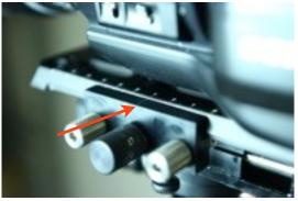
on the side to side there's a notch that got to fit with the zero balance point you've signed in the cheese plate. Once fitted this points, fasten the 2 knurled screws using the regulation key. Use a very low force in fastening those screws
