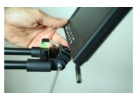
To modify the inclination of the lcd monitor fasten/ unfasten the 2 lateral screws
