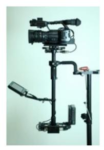
This is an example of right balanced sled. The sled doesn't fall down in any directions
