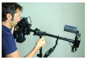
Unfasten the screw of the cilindrical knurnel handle of the gimbal and move the entire gimbal telescopically on the post. Move the gimbal right to the camcorder or right to the battery pack until the sled falls down with 2,5 seconds time of fall. Once you've regulated the right time of falling, you can center the camcorder on the side to side mouving the knobs millimetrically.
