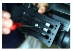
Fasten the antirotation screw for DV-HDV camcorder using the key.
