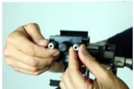
unfasten the 2 lateral locking screws on the side to side and enlarge the positioning in order to receive the cheese plate
