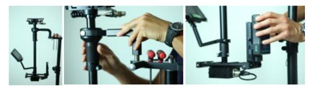
**Preparing the steadycam**Put the sled on the docking plate, positioning the gimbal handle inside the 5/8" pin of the docking plate.
