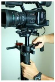
Raise up the sled from the 5/8" docking plate pin and put the sled on the other side of the docking plate, Lodging the gimbal on the fork and locking it with the security pin.
