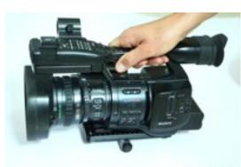
Put a perfect cilinder (for example a large felttip) under the plate in order to find the zero balance point of your camera.
